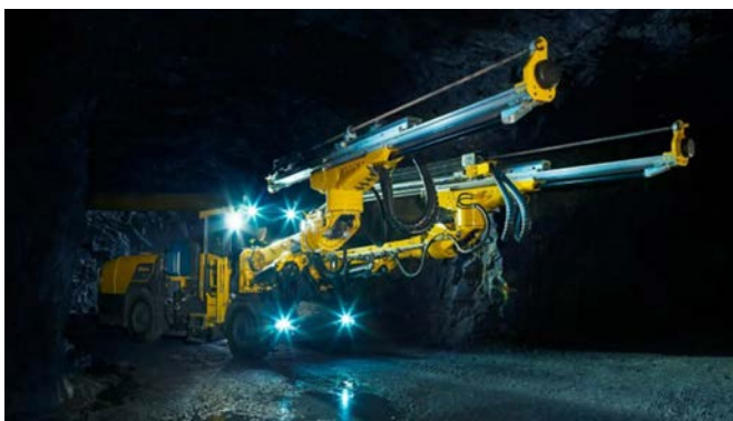
The Boomer M20 S jumbo drill rig features a hoseless boom design for fewer breakdowns, better visibility, and improved operator comfort, including a quieter cabin. It is the first rig of its kind to drill partly on battery power for cleaner, more efficient operations.
