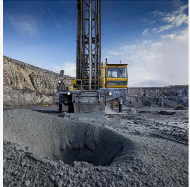
At Boliden Aitik in Sweden, Europe's largest copper mine, Epiroc Pit Viper drill rigs operate fully autonomously, enhancing safety, boosting efficiency, and reducing environmental impact. Every year, thousands of holes are drilled to extract more than 40 million tons of ore.
